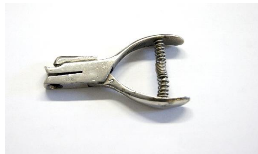
Image 2 - Pliers Obliterator, commonly used in the 60-80 times. This piece is less sophisticated, but more practical. Often integrated into the conductor's own case through a leather buckle.
